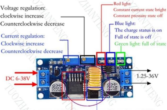
Output current: adjustable maximum 5A maximum 75W
